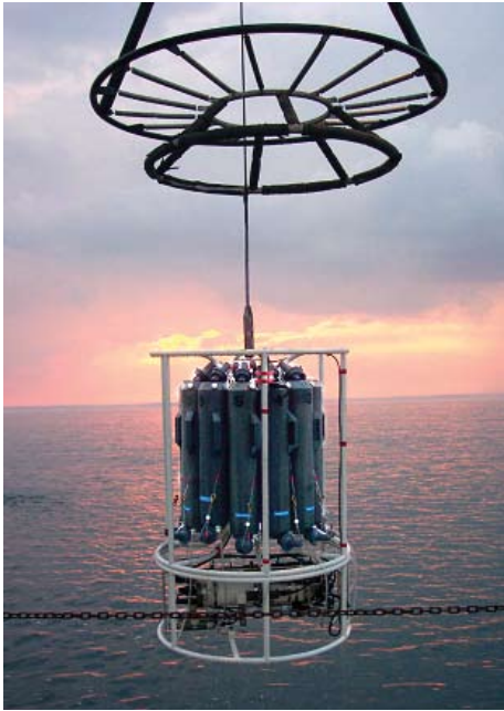
The rosette is an instrument used to collect water samples on board the R/V Peter Wise Lake Guardian . U.S. EPA GLNPO
