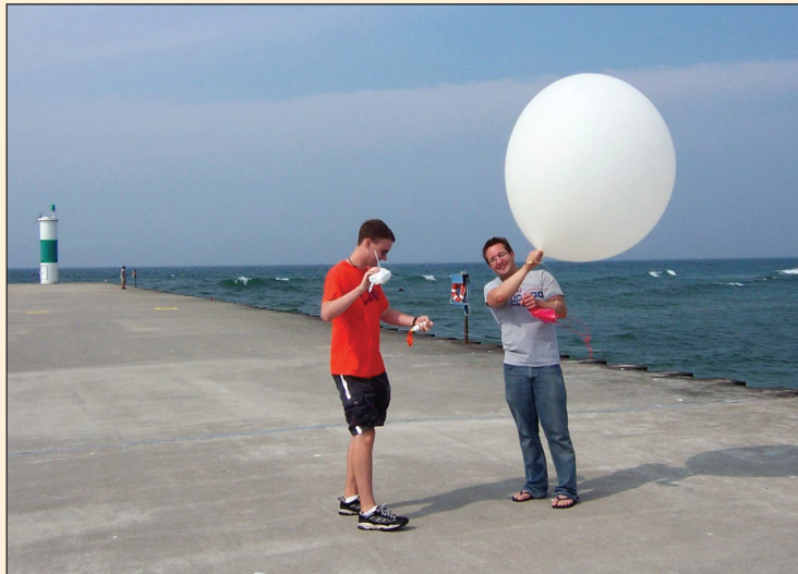
Graduate students Joe Wegman, left, and Luke Bard prepare to launch a rawinsonde near Lake Michigan.
